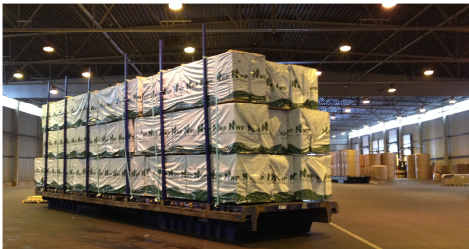
Figure 4-1 HCT Rail transport (load unit) in the Port of Göteborg. These units could be loaded onto dedicated rail wagons, is in the port transhipped by using Straddle carriers and loaded onto the ships. The loading efficiency per load unit meter is up to 80 % more
